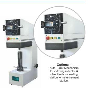
For Auto Turret Machine after clicking on cycle start button indexing mechanism will operate automatically & loading mechanism starts, once loading finishes again indexing mechanism will positioned at measuring station.
