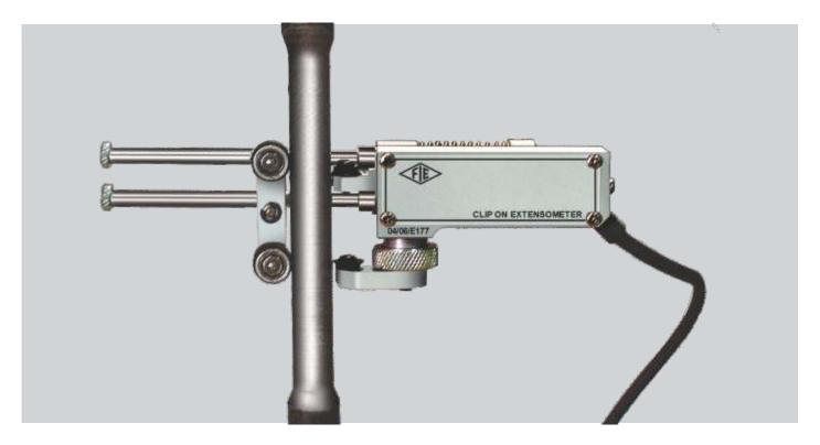
The Electronic Extensometer, Model EE-2 is manufactured as per IS:12872:1990 & ISO 9513:1989 in class 1 accuracy.
